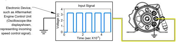
This Fuel Pump is not compatible for use with the Fuelab Electronic Fuel Pressure Regulator per Models 52901 and 52902, that creates its own pulsed signal. Refer to instructions for Electronic Regulator that may be compatible for proper wiring and installation.
