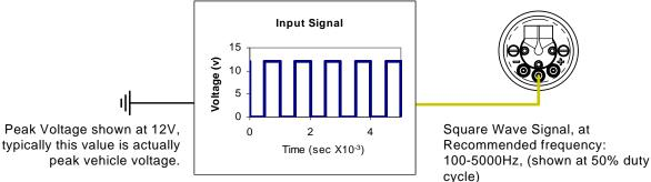
Refer to above Example 5, for use with the Fuelab Electronic Fuel Pressure Regulator, Models 52901 and 52902, that creates its own pulsed signal. These regulators automatically control the Fuel Pump, without the use of switching means or other components such as described in examples 2 and 3. Refer to instructions for the Electronic Regulator, for proper wiring and installation.
