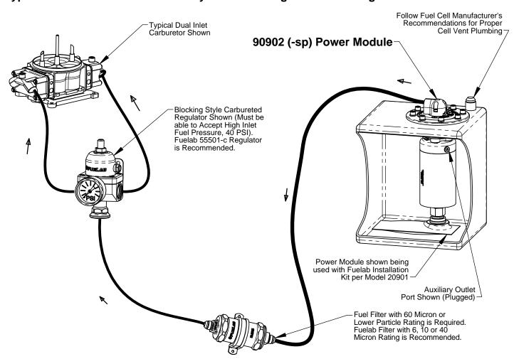
Special Note: Fuel Pump can be used with a bypass return or relief valve style regulator as well. For extended periods of operation, Fuel Pump must operate in reduced speed mode ONLY.
