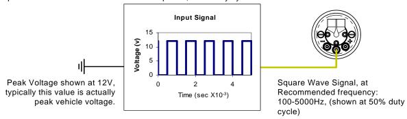
Refer to above Example 5, for use with the Fuelab Electronic Fuel Pressure Regulator, Models 52901 and 52902, that creates its own pulsed signal. These regulators automatically control the Fuel Pump, without the use of switching means or other components such as described in examples 2 and 3. Refer to instructions for the Electronic Regulator, for proper wiring and installation.
