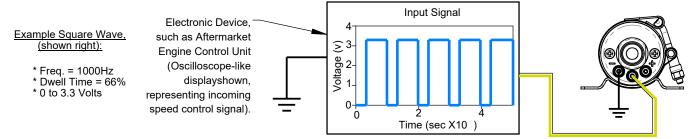
Refer to above Example 5, for use with the Fuelab Electronic Fuel Pressure Regulator, Models 52901 and 52902, that creates its own pulsed signal. These regulators automatically control the fuel pump, without the use of switching means or other components such as described in examples 2 and 3. Refer to instructions for the Electronic Regulator for proper wiring and installation.
