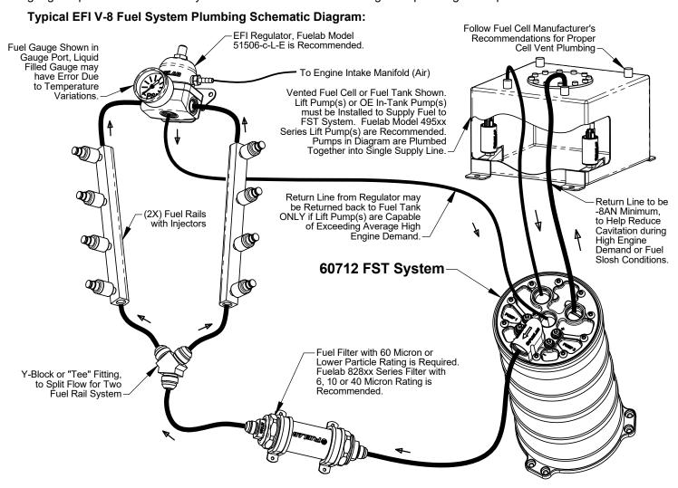
Special Note: Use in carbureted systems require a bypass return or relief valve.
