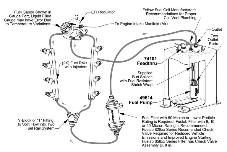
Special Note: Use in carbureted systems require a bypass return or relief valve.
