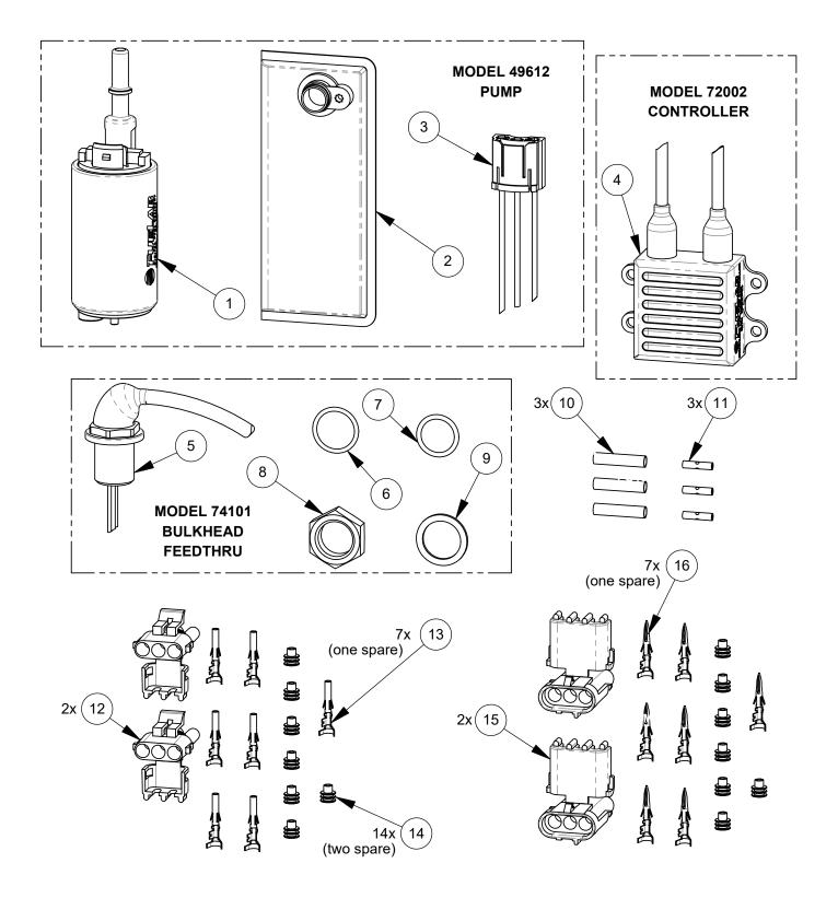
Check above diagram and list shown on previous page, to ensure no components are missing or damaged. Contact your Fuelab® distributor immediately for replacement.
