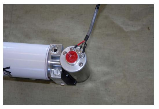
**Step 9:** The Fuel Line (Items 1 and 2) and Push-lok® fittings (PO188 and PO166) are very tight. Use a small amount of oil on the fittings and use a heat gun to soften the fuel lines slightly, to fully seat them.
