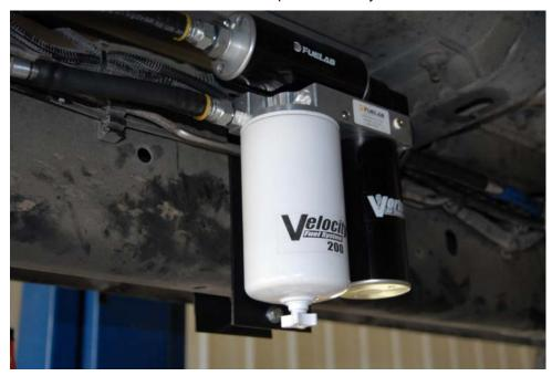
If you installed correctly you will only see a small part of the bracket and filter showing, **DO NOT** position to where the Lift Pump / Filtration System rubs against the cab body.
