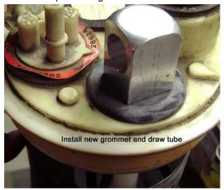
Remove and discard the original in-tank fuel pump from the fuel tank module (if present), and wire tie any wiring from pump, to secure (wiring of fuel pump is no longer required, do not short wires together). Wiring is still required for the fuel tank level sender. Remove other unneeded components within the fuel tank module as well including additional straining filters (such as shown in the photo to the left).
