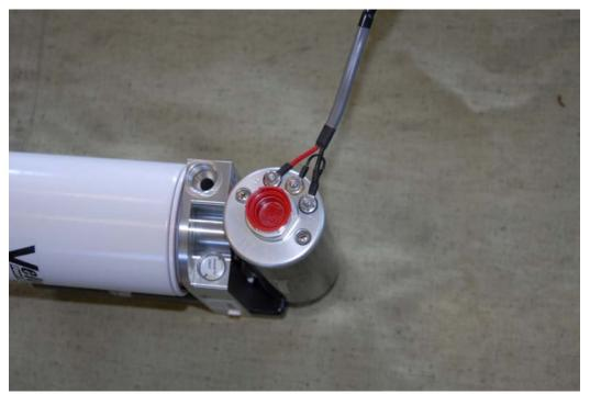
**Step 9:** The Fuel Line (items 1 and 2) and Push-lok® fittings (items 3, 4, 5, 7, 8 and 14) are very tight. Use a small amount of oil on the fittings and use a heat gun to soften the fuel lines slightly, to fully seat them.
