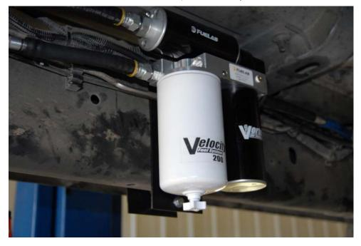
If you installed correctly you will only see a small part of the bracket and filter showing, **<u>DO NOT</u>** position to where the Lift Pump / Filtration System rubs against the cab body.
