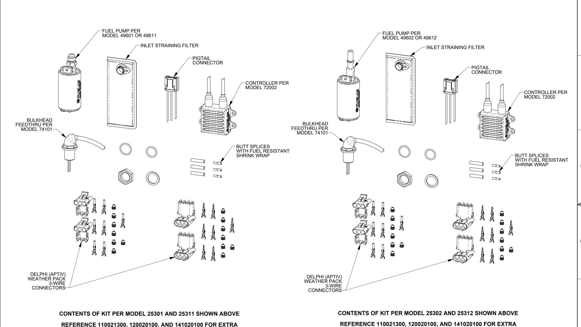
REFERENCE 110021300, 120020100, AND 141020100 FOR EXTRA DETAILS INCLUDING DIMENSIONS, PERTAINING TO INCLUDED MODELS DETAILS INCLUDING DIMENSIONS, PERTAINING TO INCLUDED MODELS
